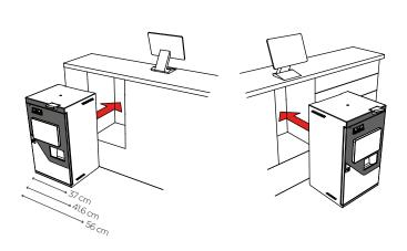
Compact design for easy installation on the workbench, both on the operator and on the customer side
