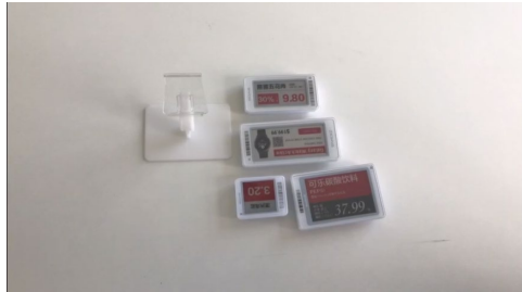
The ESL tag slots into Installation fixture
