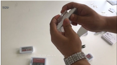
The installation of bulk ESL clip is relatively simple. Put the labels in Clip.
